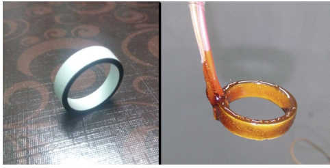
Fig. 1: Piezo-ceramic Transducer without coating (left) and with coating (right)
